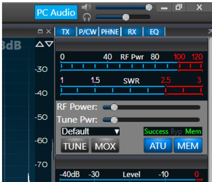
If you want to re-check the 'tune' at any point, you can hit the 'TUNE' button (it's a persistent switch - i.e. manually click to turn on, manually click again to turn off).
