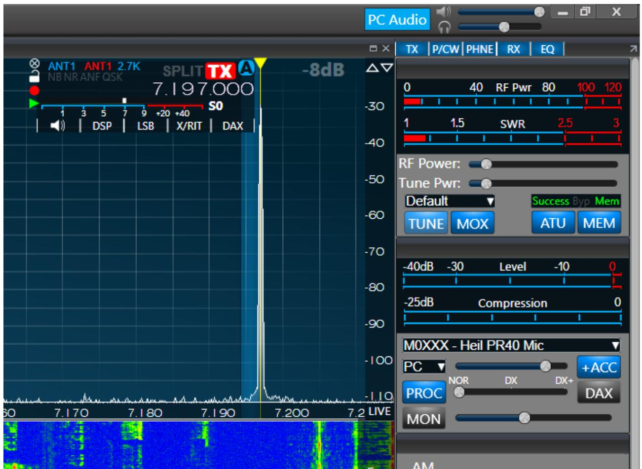
The 'MOX' button operates just like the 'TUNE' button. Click on/Click off - it's not auto-release like some software implemented 'PTT' type switches where you have to hold it on. Obviously this is where your microphone becomes active and you're on the air.
